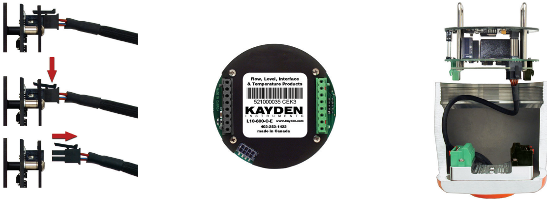
Figure 10 - Disconnecting Sensor Connector from the Electronics Module
